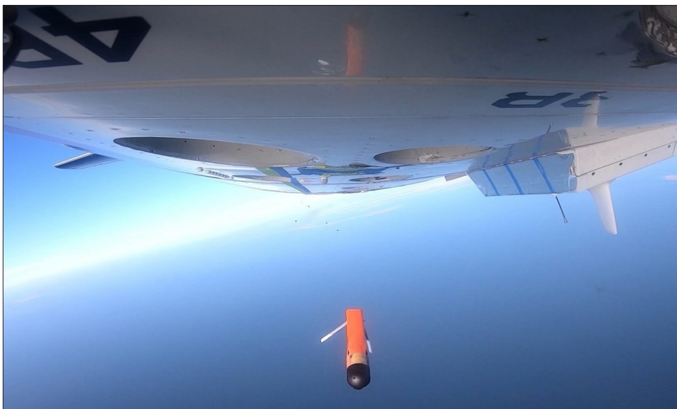
An Altius-600 small uncrewed aircraft system deployed in the eye of Hurricane Ian from NOAA's P-3 Hurricane Hunter aircraft collected observations from the lower altitudes of Ian, measuring wind speeds as strong as 216 mph at 2150 feet above the ocean. Photo credit: NOAA.
