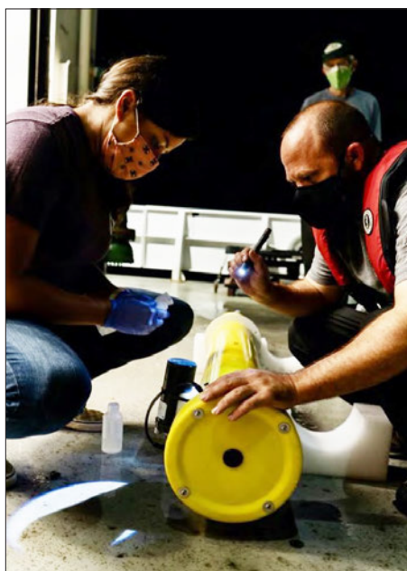
AOML scientists Emily Osborne and Andy Stefanick prepare a biogeochemical Argo profiling float for deployment in the Gulf of Mexico. Photo credit: Grace Owen, University of Miami.
