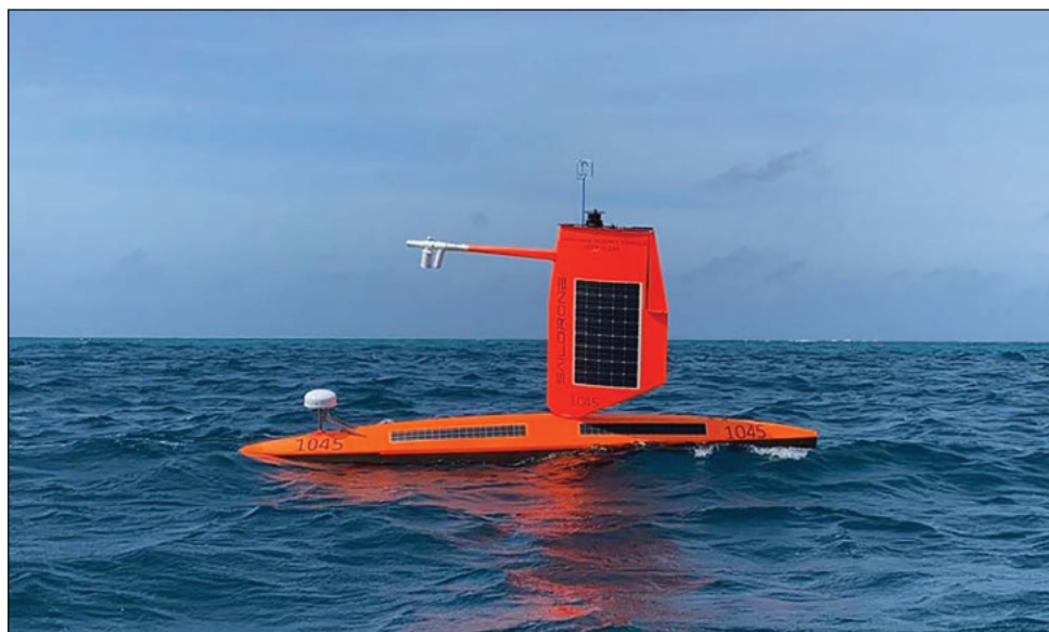
Saildrone 1045 made history in September when it became the first uncrewed surface vehicle to collect observations from inside the eye of a hurricane. A specially-designed hurricane wing enabled the 23-foot drone to withstand the extreme winds and chaotic sea state encountered in Hurricane Sam. Video footage from an onboard camera can be viewed at https://www.noaa.gov/news-release/world-first-ocean-drone-captures-video-from-inside-hurricane .
