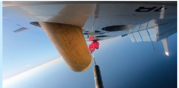
An ALAMO profiling float is deployed from a NOAA P-3 Hurricane Hunter aircraft.
