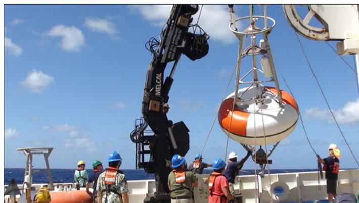
The Brown's deck crew, PMEL's mooring technicians, and AOML volunteers deploy a PIRATA buoy at 15°N, 38°W.
