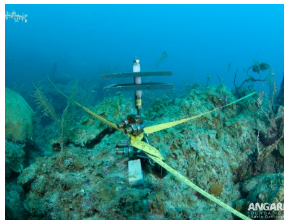
Figure 6: CAU and BMU pair deployed during the expedition. CAUs are two parallel PVC plates to quantify settled accretors. BMU is mounted coral skeleton installed at the base of the metal stake and has been encrusted.
