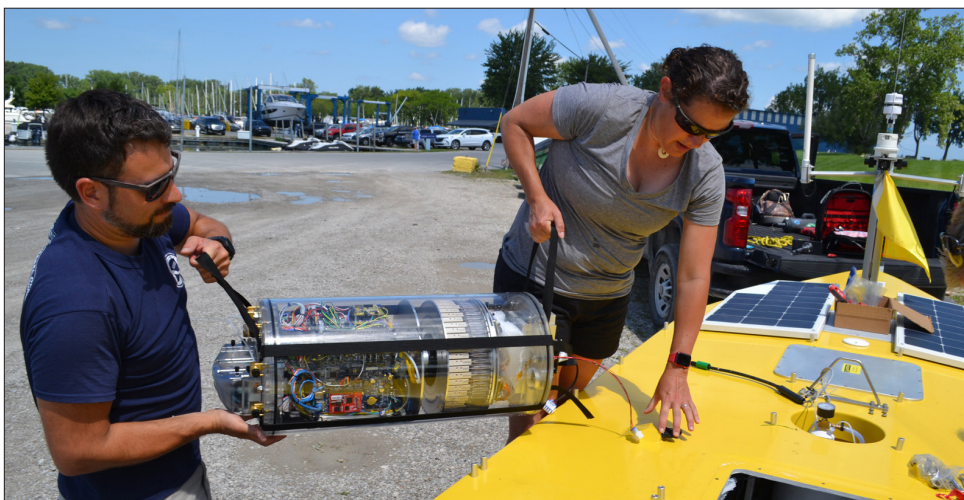
NOAA-GLERL marine engineer Kyle Beadle and scientist Reagan Errera, PhD, remove MBARI’s 3G ESP sampling instrument from the inside of the SeaTrac autonomous platform. Image credit: NOAA-AOML.
