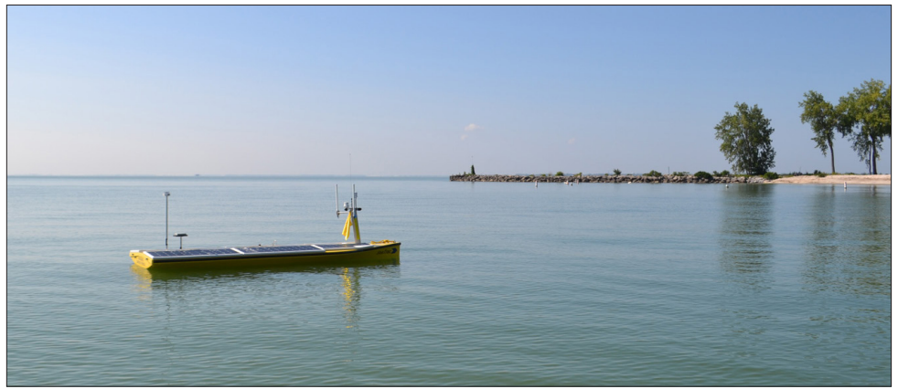
The solar-powered SeaTrac autonomous surface vehicle, roughly the shape of a stand up paddle board, successfully sampled the shallow waters of western Lake Erie. Image credit: NOAA-GLERL
