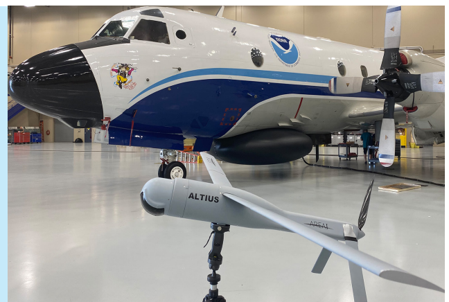
The Altius-600 UAS (foreground) was deployed from NOAA’s P-3 aircraft (background), transmitting data from Tammy at altitudes as low as 940 feet above the ocean surface. Image credit: NOAA-AOML
