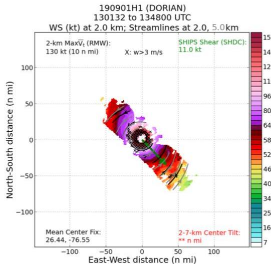
*Figure 1: Analysis coverage degradation in the eyewall region due in part to rapid changes in crab angle entering and exiting the small eyewall (RMW ~ 18 km) of Hurricane Dorian (2019).*
