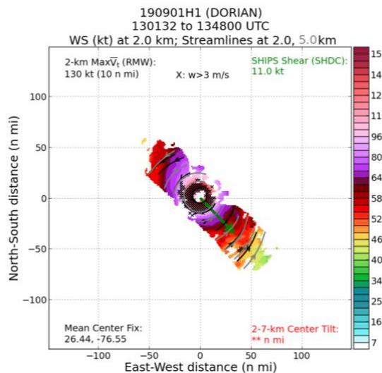
*Figure 1: Analysis coverage degradation in the eyewall region due in part to rapid changes in crab angle entering and exiting the small eyewall (RMW ~ 18 km) of Hurricane Dorian (2019).*
