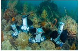
*Figure 3:* Submerged Automated Samplers (SAS) deployed to collect water samples every 3 hours.
