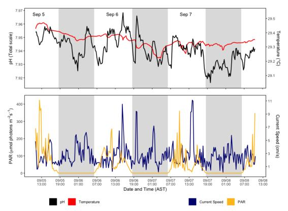
**Figure 4**: Data from the Salt River Bay diurnal suite monitoring from Sept 5th to Sept 8th. Top panel: pH and temperature from SeaFET. Bottom panel: Photosynthetically Available Radiation (PAR) and current speed from EcoPAR and Tiltmeter. Grey blocks denote night time throughout sequence of the plot. Instruments measured parameters every 15 minutes.
