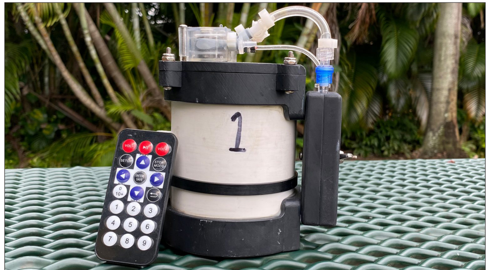
The Subsurface Automated Environmental DNA Sampler designed at AOML provides the science community with a low-cost option for filtering and collecting DNA from water samples.
