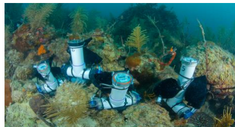
Deployed SAS for collecting water samples every three hr. Picture Credit: Kevin Davidson.
