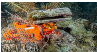
A CAU (the two, parallel plates) and a BMU (not readily visible, though located at base of stake) before retrieval. These instruments were left in the field for three years to estimate accretion and bioerosion, respectively. Picture Credit: Kevin Davidson.
