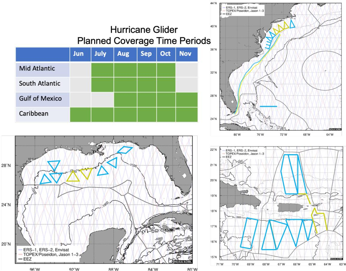
**Figure 1.** Planned transects of NOAA supported glider observations (blue), and lines of potential glider trajectories using requested Naval Oceanographic Office gliders (yellow).
