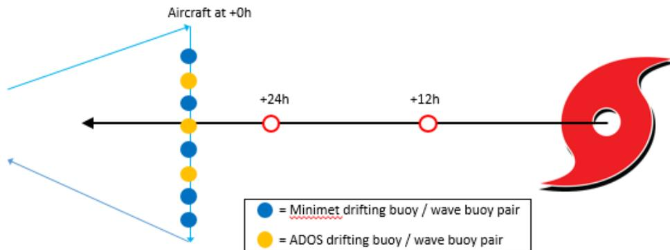
**Figure 3.** A-sized DWSB drifters. Representative deployment line of drifter pairs 24h ahead of the arrival of gale-force winds, from a C-130J.
