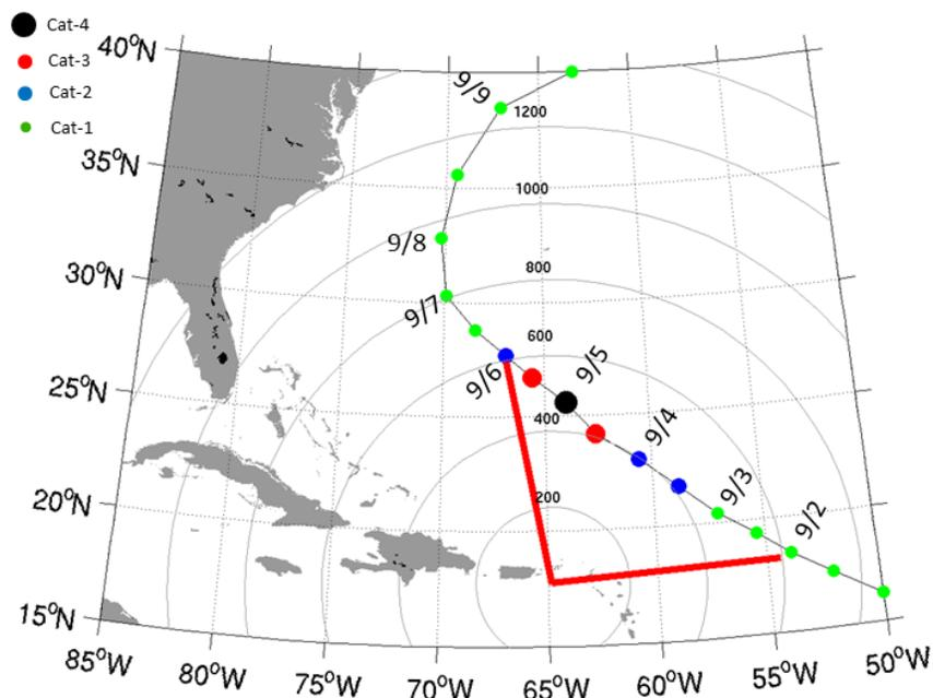
**Figure OC-1:** Storm track with locations plotted every 12 hours. Range rings are 200 n mi relative to the forward operating base at St. Croix, USVI (STX/TISX), and the red line delineates storm locations within 600 n mi of STX. In this example, the storm center remains within 600 n mi for 4 days.
