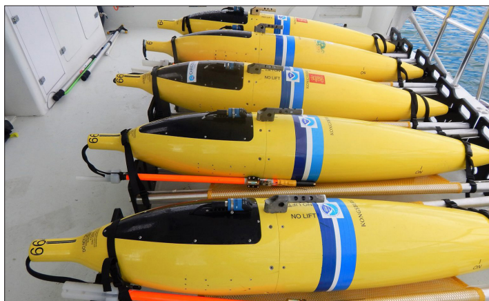
Hurricane gliders safely retrieved and on deck after having spent much of the 2020 Atlantic hurricane season at sea. Credit: NOAA AOML.
