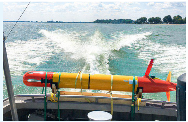
A long range autonomous underwater vehicle is ferried to the western basin of Lake Erie to test its ability to detect and measure toxic algal blooms.
