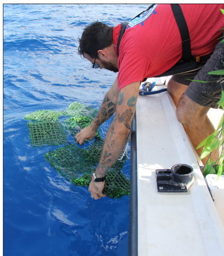
AOML researchers created and deployed GPS tracked Sargassum-simulating drifters in the tropical Atlantic Ocean and Caribbean Sea in 2018. These experiments provided valuable information on how wind and ocean currents affect the transport and distribution of Sargassum.
