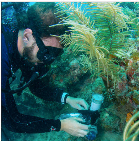
Nathan Formel, a Cooperative Institute research associate at AOML, deploys a Subsurface Automated Sampler to monitor temperature and carbonate chemistry changes at a reef in the Florida Keys.
