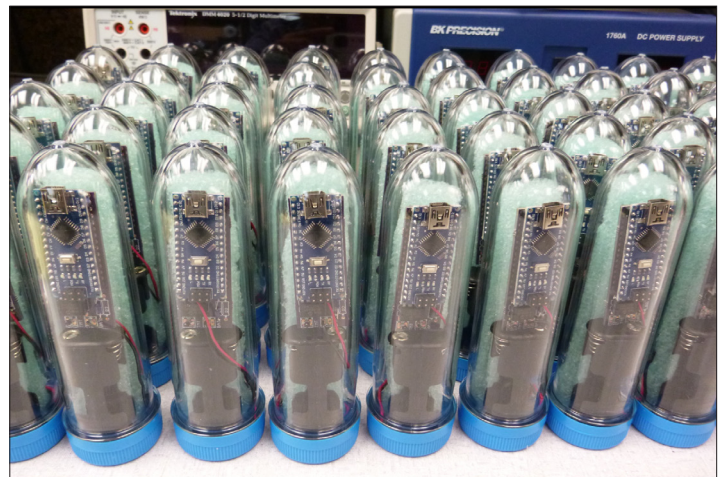
The diminutive AOML-designed temperature sensor, assembled for about $9 in parts, will be deployed at coral reef sites throughout the Caribbean Sea, Atlantic Ocean, and Indo-Pacific through a partnership with Reef Check Foundation.
