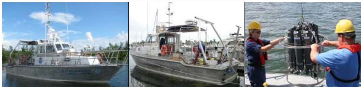
Figure 4. Left: R/V Hildebrand forward view. Middle: aft view showing A-frame. Right: Seabird rosette and CTD being deployed from the Hildebrand by NOAA scientists C. Featherstone and LT. R. Kotkowski.
