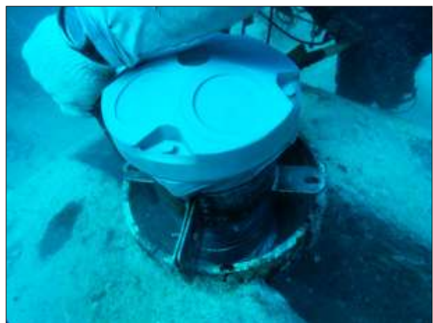
Figure 7. Mount with ADCP instrument.
