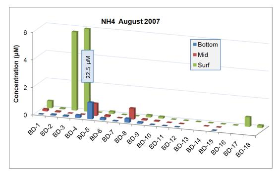
Figure 15: August 2007 ammonium concentrations for the Boynton-Delray water quality monitoring stations.
