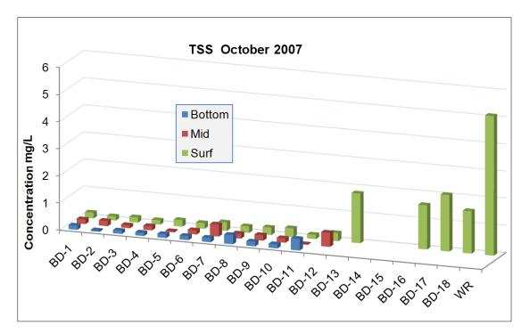
Figure 28: October 2007 total suspended solids concentrations for the Boynton-Delray water quality monitoring stations.
