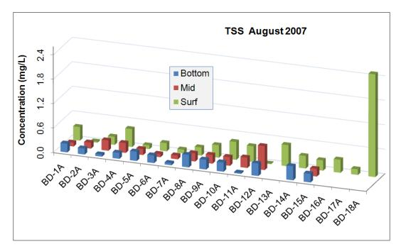
Figure 13: August 2007 total suspended solids concentrations for the Boynton-Delray water quality monitoring stations.
