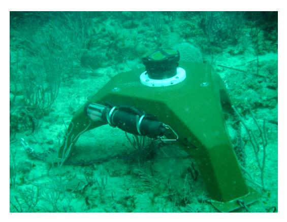
Figure 133: Photograph of the acoustic Doppler current profiler unit installed on the Gulf Steam Reef (south), operational beginning September 29, 2006.
