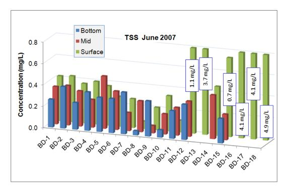
Figure 5: June 2007 total suspended solid values for the Boynton-Delray water quality monitoring stations.
