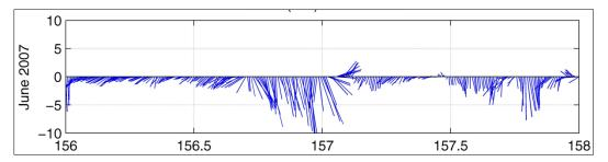
Figure 134b: Wind direction and velocity data from buoy LKWF1 during the time of the June 2007 cruise. Length of each stick is proportional to the wind speed (m/s) as given by the y-axis (arrows point to the direction the wind is coming from).
