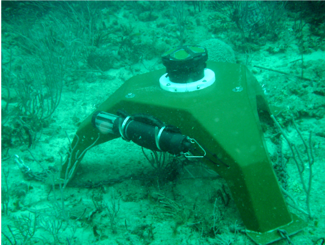
Figure 133: Photograph of the acoustic Doppler current profiler unit installed on the Gulf Stream Reef (south), operational beginning September 29, 2006.
