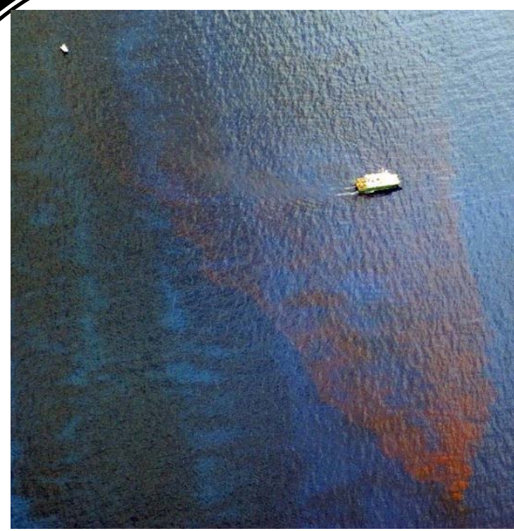
Image of rhodamine dye from the South Central wastewater outfall, Palm Beach County, Florida, July 2008. Vessel shown is R/V F.G. Walton-Smith conducting tracer study for NOAA FACE program.
