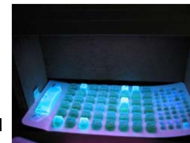
Image of Enterolert Quanti tray under UV lamp. Fluorescent wells indicate specific presence of enterococci.
