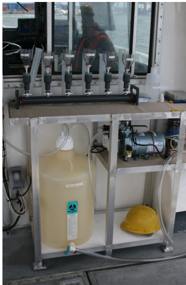
Figure 3. Work table installed aft of cabin, for immediate filtration of samples and for storage.
