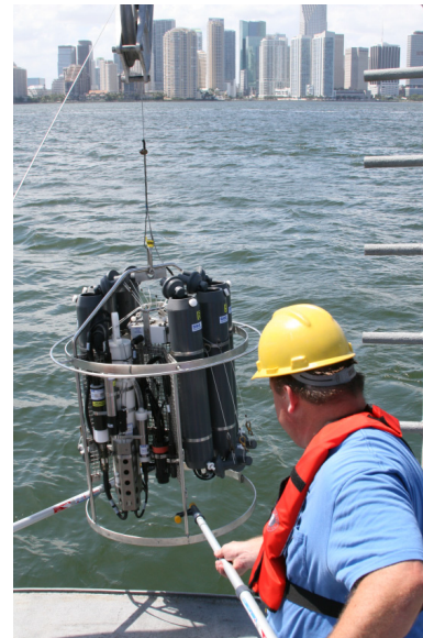
Figure 4. Seabird CTD/rosette during a test of the system, being brought on board the Hildebrand by C. Featherstone.
