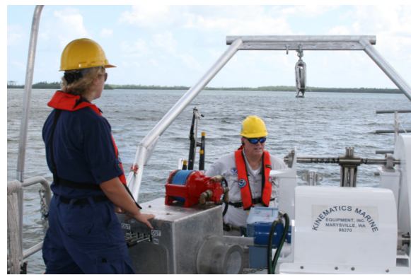
Figure 2. New A-frame, winch, and hydraulic controls undergoing sea trials.
