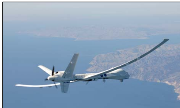
Fig. 8.2 In FY 2006, NOAA, NASA, and a private sector firm successfully evaluated the potential for Unmanned Aerial Systems (UAS) to meet NOAA operational needs. The Altair UAS was used to carry a variety of sensors including the Digital Camera System (DCS) and Electro-Optical Infrared (EO/IR) Sensor to demonstrate how operational needs of NOAA could be met in future UAS flights. The DCS was used in shoreline mapping and in along-shore/inland feature characterization for habitat mapping/ ecosystem monitoring. The EO/IR system was used for fisheries surveillance and marine mammal surveys.
