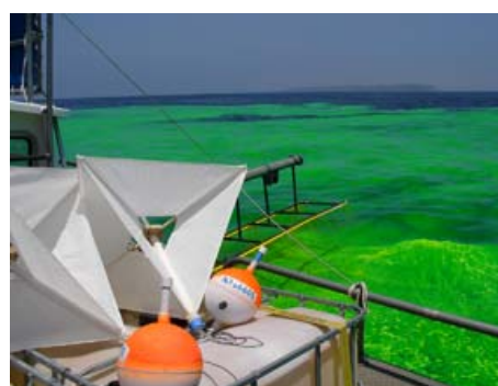
Fig 8.5 Building on capabilities developed in the recent past, a fluorescein dye solution, mixed to a density and concentration to simulate a dispersed oil plume, was deployed during the 2006 Safe Seas exercise. The horizontal and vertical micro-scale movements of water were successfully measured, supplying needed data that will improve 3-D modeling capabilities and will refine the protocol for monitoring dispersed oil.
