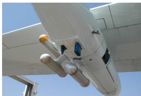
Fig. 8.3 An aircraft-based water vapor sensor was successfully field tested in 2005-2006 on commercial aircraft. Results of the test were presented at the American Meteorological Society Conference in 2006. Increased observations from sensors deployed using aircraft of opportunity will support improvements to numerical models used in NOAA products and services.
