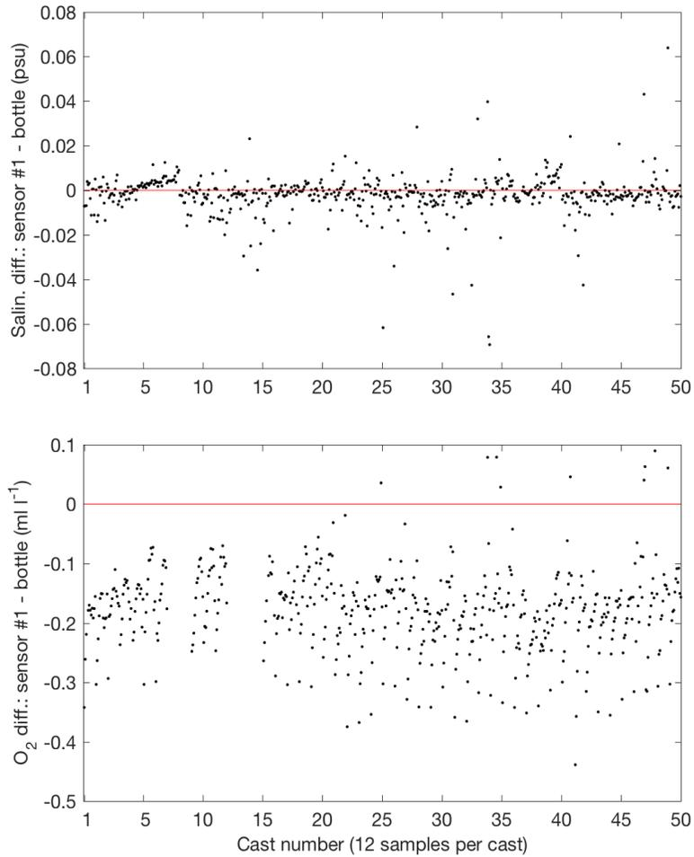
**Figure 3** (top) Difference between salinity value from CTD primary sensor and bottle sample. Negative values indicate that bottle sample was higher than sensor value. Red line shows a difference of zero. (bottom) Same as (top) except for oxygen concentration.
