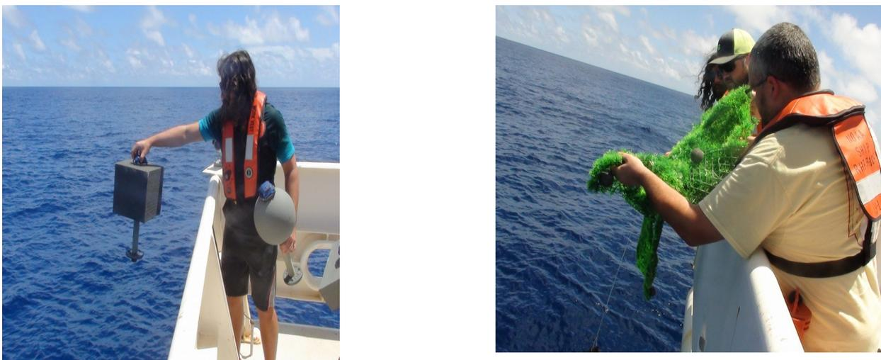
Figure 5 Deployments of (left) debris drifters and (right) sargassum drifters at 0°, 23°W.
