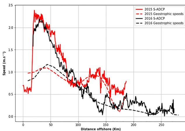
**Figure 4.** A comparison of the 2015 (red) and 2016 (black) dedicated ship acoustic Doppler current profiler (S-ADCP) transects with the cross-track satellite-derived geostrophic velocities from the same day (dashed).
