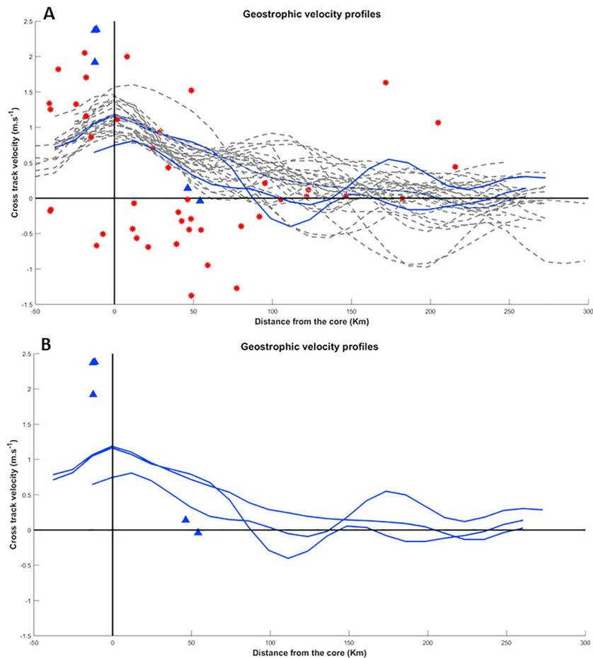
**Figure 3.** (a) Cross-track surface geostrophic velocity (m/s) relative to the velocity maxima of the Agulhas Current. A positive velocity indicates a southwest direction. The blue triangles (red stars) indicate the position and velocity of the drifters that leaked into the South Atlantic Ocean (remained in the Indian Ocean) crossed the transect. Subplot (b) highlights the cross track geostrophic velocities and drifter velocities for the drifters that leaked into the South Atlantic Ocean.
