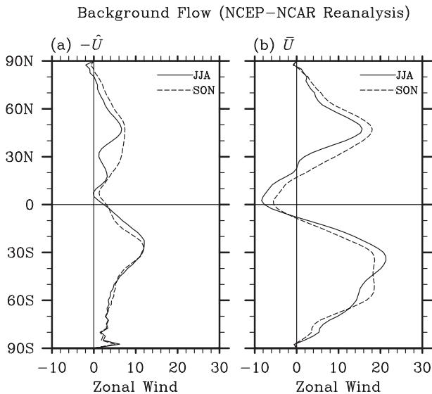
FIG. 10. The background mean zonal winds ( $\text{m s}^{-1}$ ) from the NCEP–NCAR reanalysis in JJA and SON: (a) the background vertical zonal wind shear  $-\tilde{U}$  and (b) the background vertical zonal wind mean  $\bar{U}$ . The background mean states are calculated by the zonal average between  $120^\circ$  and  $40^\circ\text{W}$  as  $\tilde{U} = (U_{750\text{mb}} - U_{250\text{mb}})/2$  and  $\bar{U} = (U_{750\text{mb}} + U_{250\text{mb}})/2$ .
