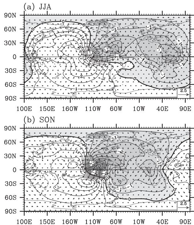
FIG. 5. The 200-mb velocity potential ( $10^6 \text{ m}^2 \text{ s}^{-1}$ ) and divergent wind ( $\text{m s}^{-1}$ ) difference between the LAWP and SAWP CAM3 ensemble runs in (a) JJA and (b) SON. The negative velocity potential difference is shaded and the contour interval is  $0.5 \times 10^6 \text{ m}^2 \text{ s}^{-1}$ .
