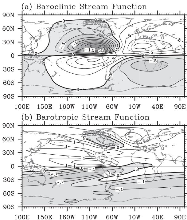
FIG. 14. Streamfunctions ( $10^7 \text{ m}^2 \text{ s}^{-1}$ ) of the (a) baroclinic and (b) barotropic components in JJA from the simple model run:  $\bar{U} = 0$  (without the background vertical wind mean) over the Southern Hemisphere. The negative streamfunction is shaded. The contour interval in (a) is  $0.25 \times 10^7 \text{ m}^2 \text{ s}^{-1}$  and the contour interval in (b) is  $0.05 \times 10^7 \text{ m}^2 \text{ s}^{-1}$ .
