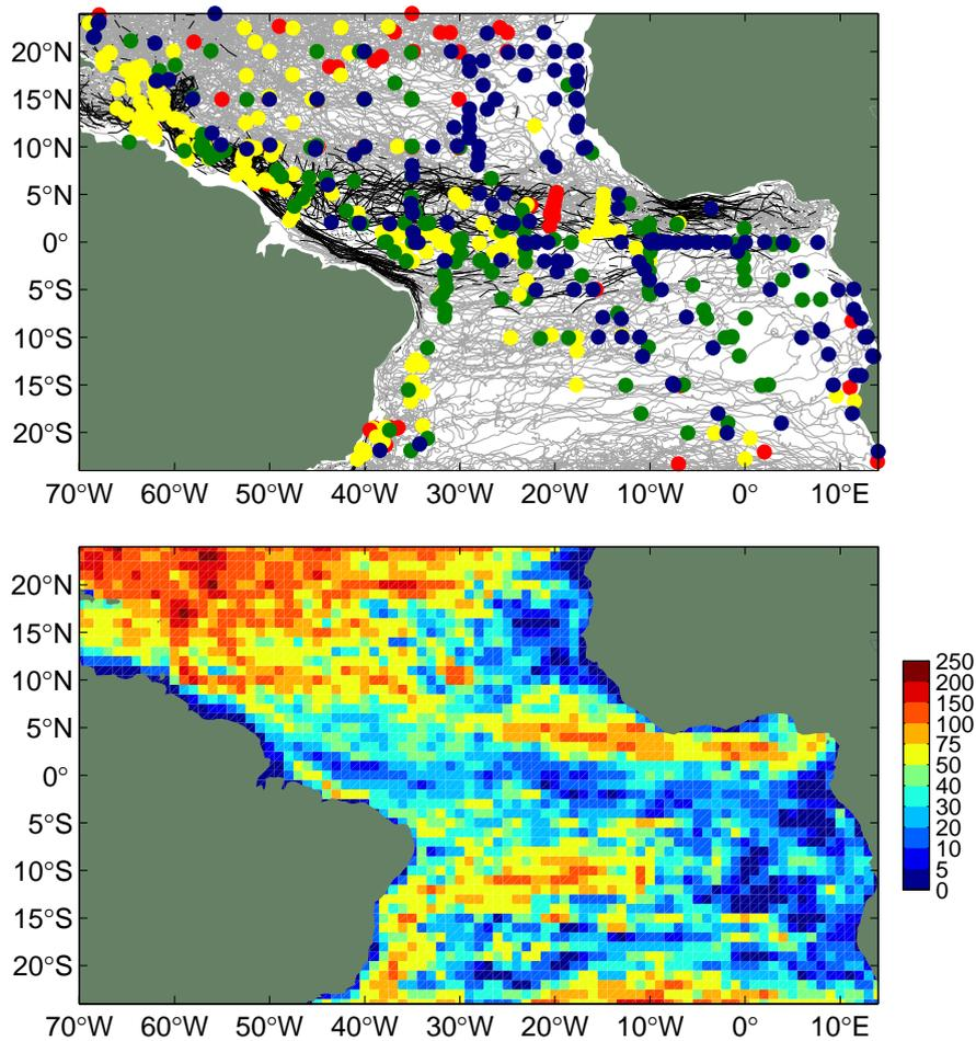
Fig. 2. *Top*: Trajectories of drifters moving at speeds  $< 50\text{ cm/s}$  (light gray) and faster (black). Deployment locations are indicated by colored bullets: 1990–1997 (red), 1998–1999 (yellow), 2000–2001 (green) and 2002–February 2004 (blue). Some recent deployments overlay older ones. *Bottom*: Density of observations (drifter days per square degree).
