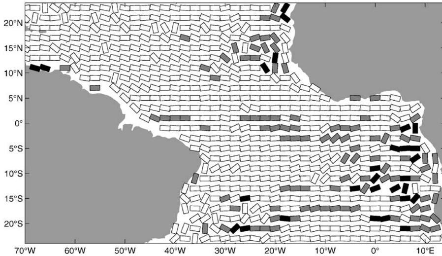
Fig. 5.  $2^\circ \times 1^\circ$  bins used to average drifter observations. Bin orientation is set by a principle component analysis of the velocity variance. Every other bin on the  $1^\circ \times 1^\circ$  grid is shown. Unshaded bins contain  $>20$  observations per square degree; gray bins contain 5–20 observations; black bins contain  $<5$  observations.
