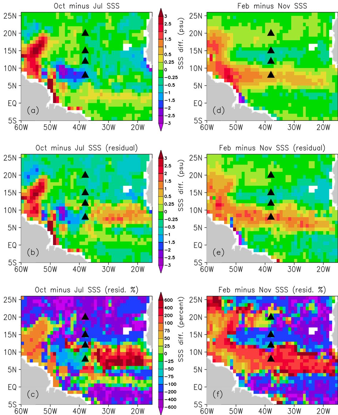
**Fig. 5** (a) Difference between SSS in October 2012 and July 2012. (b) Same as (a) except SSS due to horizontal advection. (c) Same as (a) except percentage of SSS change that is due to horizontal advection. Positive values in (c) indicate an increasing tendency of SSS due to advection, negative values a decreasing tendency. (d)–(f) Same as (a)–(c) except difference between February 2013 and November 2012.
