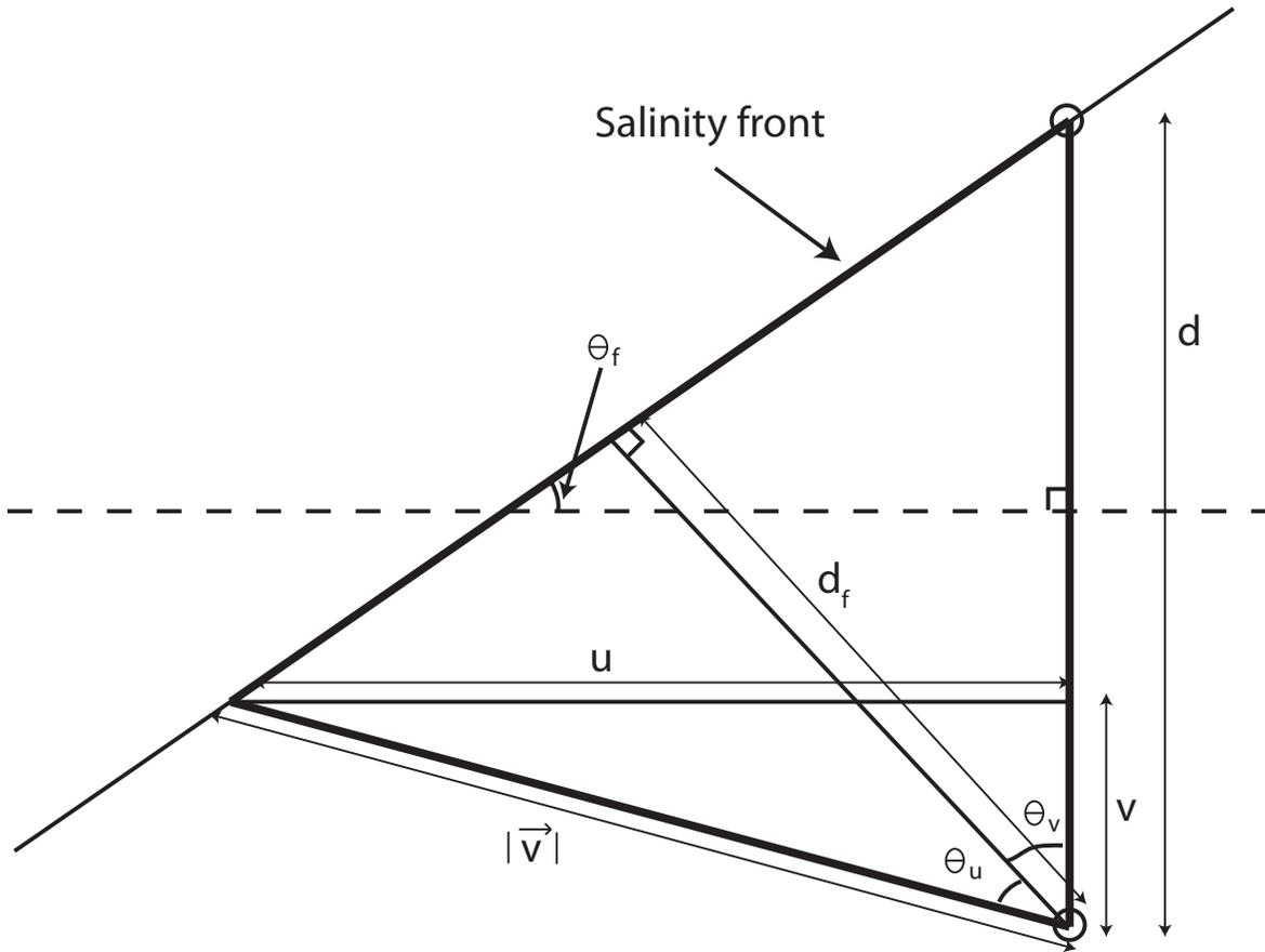
**Fig. A1** Diagram illustrating the methodology used to calculate the angle between the low-salinity front and a line of constant latitude ( $\theta_f$ ). Black circles indicate positions of PIRATA moorings, and  $u$  and  $v$  are observed zonal and meridional velocity, respectively, averaged between the moorings.
