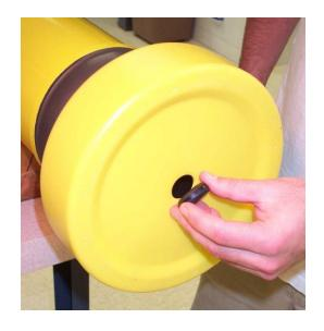
5) Start a Manual or Pressure Activated Deployment as described above in the "Manual Deployment with the Reset Tool" and "Pressure Activation Deployment" sections. This will trigger the Mission Activation self tests. Where applicable, the description below indicates where the two versions of the self tests differ.
