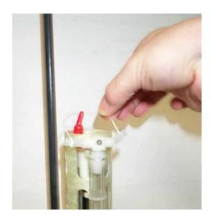
4) Carefully remove the black rubber plug from the bottom center of the yellow cowling as shown in the image below. This will allow you to verify air bladder inflation in the steps below. **Use only your fingers to remove**
