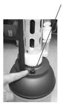
rotate counter -clockwise to unscrew plug.
