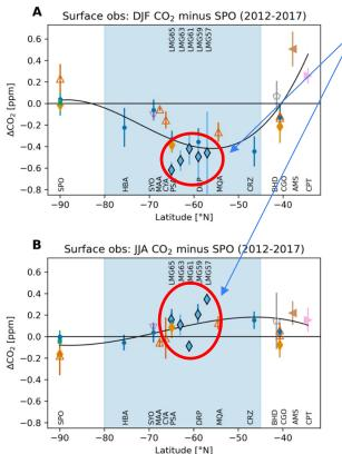
Measurements from ships quality comparable to Surface Monitoring Stations and Aircraft Campaigns.
