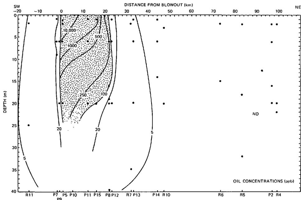
Figure 2. Concentrations of oil along a transect oriented to the northeast of the IXTOC-1 blowout, September 1979 (after Fiest and Boehm, 1980).
