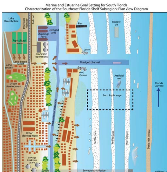
Figure 9. Southeast Florida coast integrated conceptual ecosystem model—plan view diagram.
