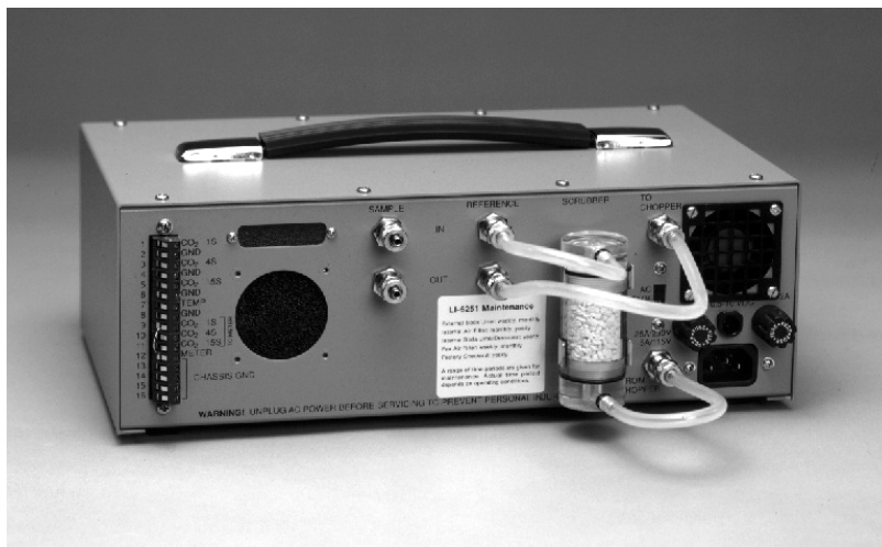
Figure 2-2. Hose connections for operation in absolute mode.
