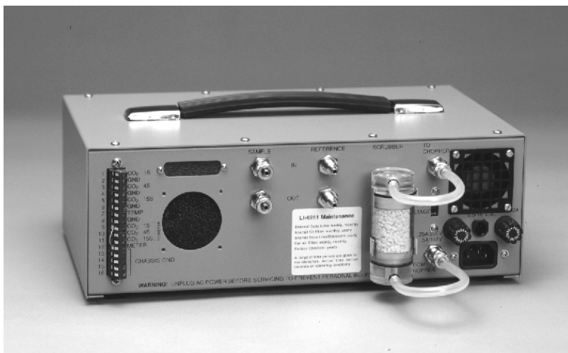
Figure 2-1. Hose connections for operation in differential mode.
