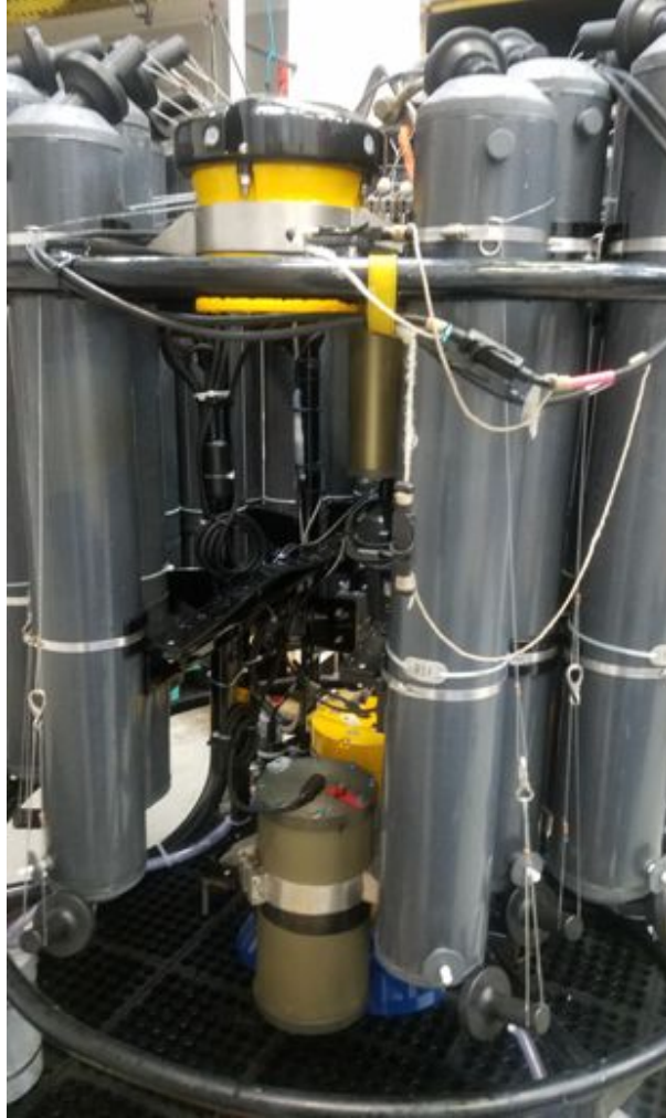
Figure 19. Instruments and battery pack on rosette. UVP is not mounted in this photo.
