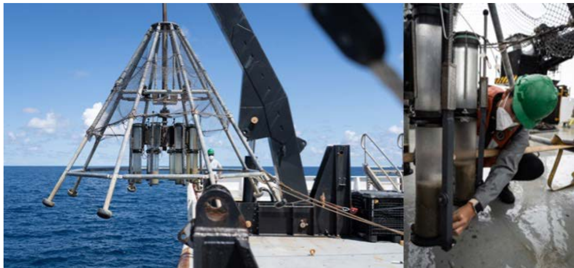
Figure 1: Sediment corer safely recovered after being deployed to 3,200 m (left), and Dr. Emily Osborne (AOML/NOAA, right) checking the integrity of the cores after recovery of the instrument. Photo credit: Grace Owen (University of Miami).
