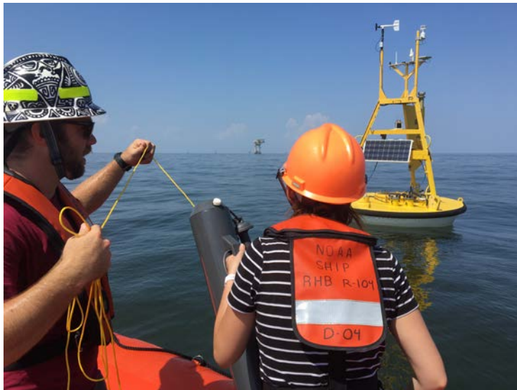
Picture 1. Small boat operation to deploy a hand-held Niskin as close to the OA buoy as possible to collect validation samples.
