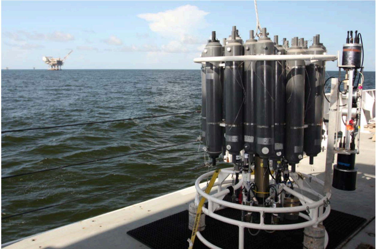
Picture of the fantail of the Brown off the coast of Mississippi with oil rigs in the background Wednesday Jul 24. The CTD with Niskin bottles and pH profiler strapped to the side is in the foreground. (courtesy Andrew Margolin)
