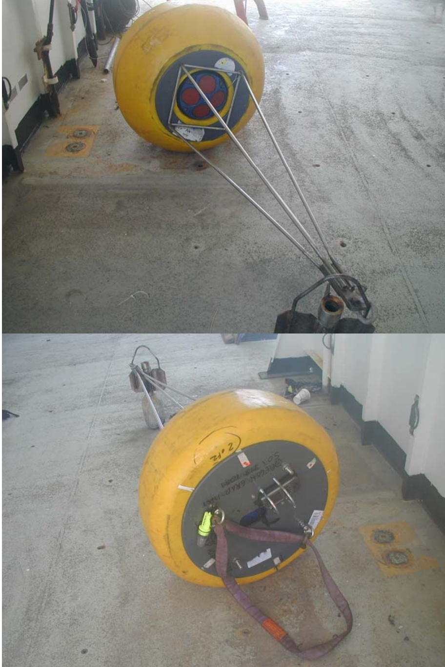
Figure 2: Photos showing the ADCP transducers (top), buoy, and GPS (lower picture, just right of center).
