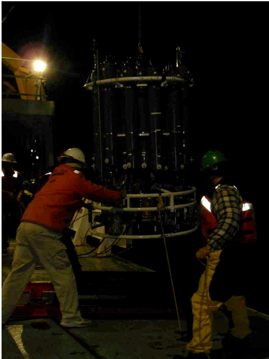
Figure 1: We are not in the tropics anymore. Deployments and sampling have become more challenging with rough seas and falling temperatures. Shown is a nighttime recovery of the CTD/O2 package. The key is to prevent the 2000 lbs. package from swinging like a pendulum
