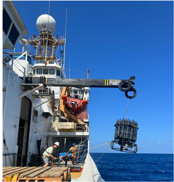
A CTD being recovered on the last day of science operations. Photo credit: Alex Fine (AOML)
