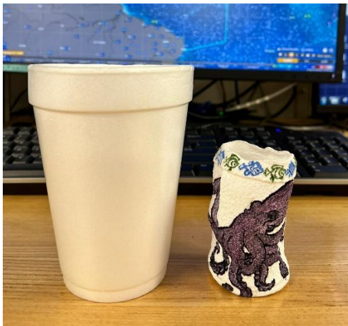
Comparison of a normal Styrofoam cup (left) and a cup that has been decorated and sent to 3160 m. (right).
