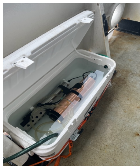
Makeshift ambient seawater bath for a prototype sensor. Seawater runs from an inline system in the main lab to the instrument sitting on the back deck, from the instrument into the container, and then drains from the hose near the top into the ocean. Photo credit: Zach Erickson.
