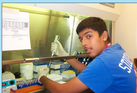
High school student intern Aditya Shetty loads samples into a real-time qPCR instrument to test for a human fecal genetic marker.
