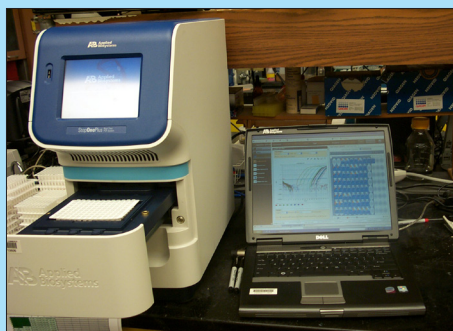
A qPCR (quantitative real-time polymerase chain reaction) instrument at AOML is used to amplify and detect targeted DNA molecules.
