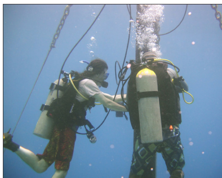
AOML's Mike Jankulak and Gordon Walker from PacIOOS install a CTD (conductivity-temperature-depth) sensor along the CREWS pylon.
