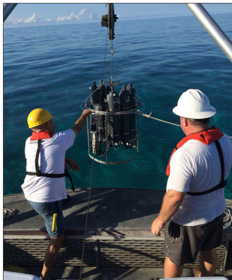
Jack Stamates and Charles Featherstone of AOML deploy a CTD instrument with Niskin water sampling bottles to measure physical ocean parameters and collect water for nutrient, microbial, and metagenomic analyses.
