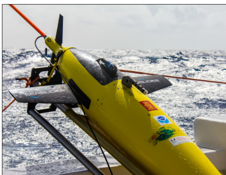
A NOAA/AOML-CARICOOS underwater glider ready for deployment in the Caribbean Sea. The gliders are remotely operated and navigate under harsh ocean conditions, including hurricane-force winds.
