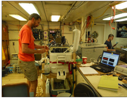
Kevin Sullivan of AOML works to measure the fugacity of carbon dioxide in water column samples gathered during leg 1. Photo courtesy of Rachel Shelley.
