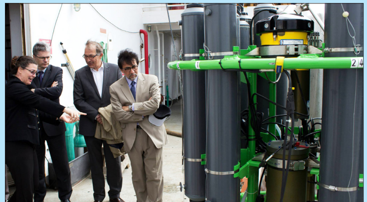
Molly Baringer of AOML explains to the Brown's distinguished guests how scientists use a CTD/O 2 (conductivity-temperature-depth-oxygen) water sampler package lowered via cable into the ocean to gather data about the physical and chemical properties of the water column.
