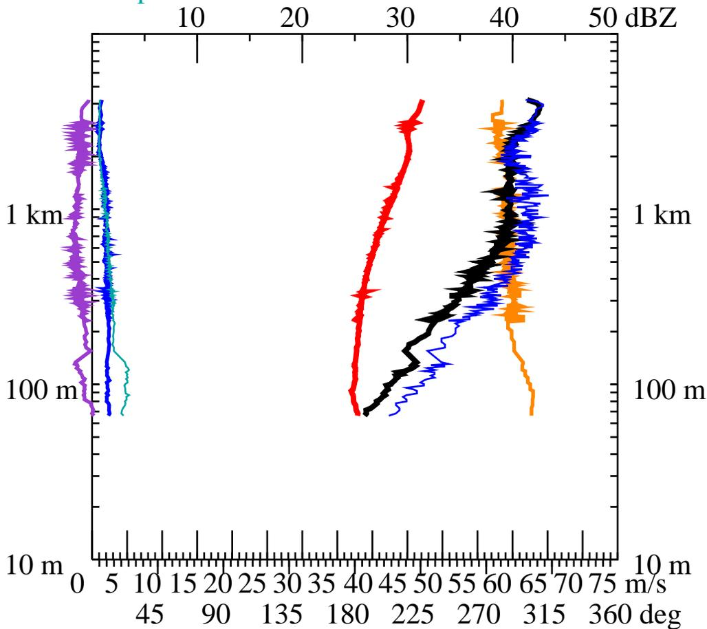
**Figure 4. Vertical profile of horizontal winds at 1150 UTC, 24 October 2005, estimated by the Velocity-Azimuthm Display method. Winds were calculated in rings from 5 to 12 km from the Miami WSR 88D at tilt angles from 0.5 to 19.5 degrees. Values are plotted on a logarithmic scale to accentuate the structure below the 1 km height.**
