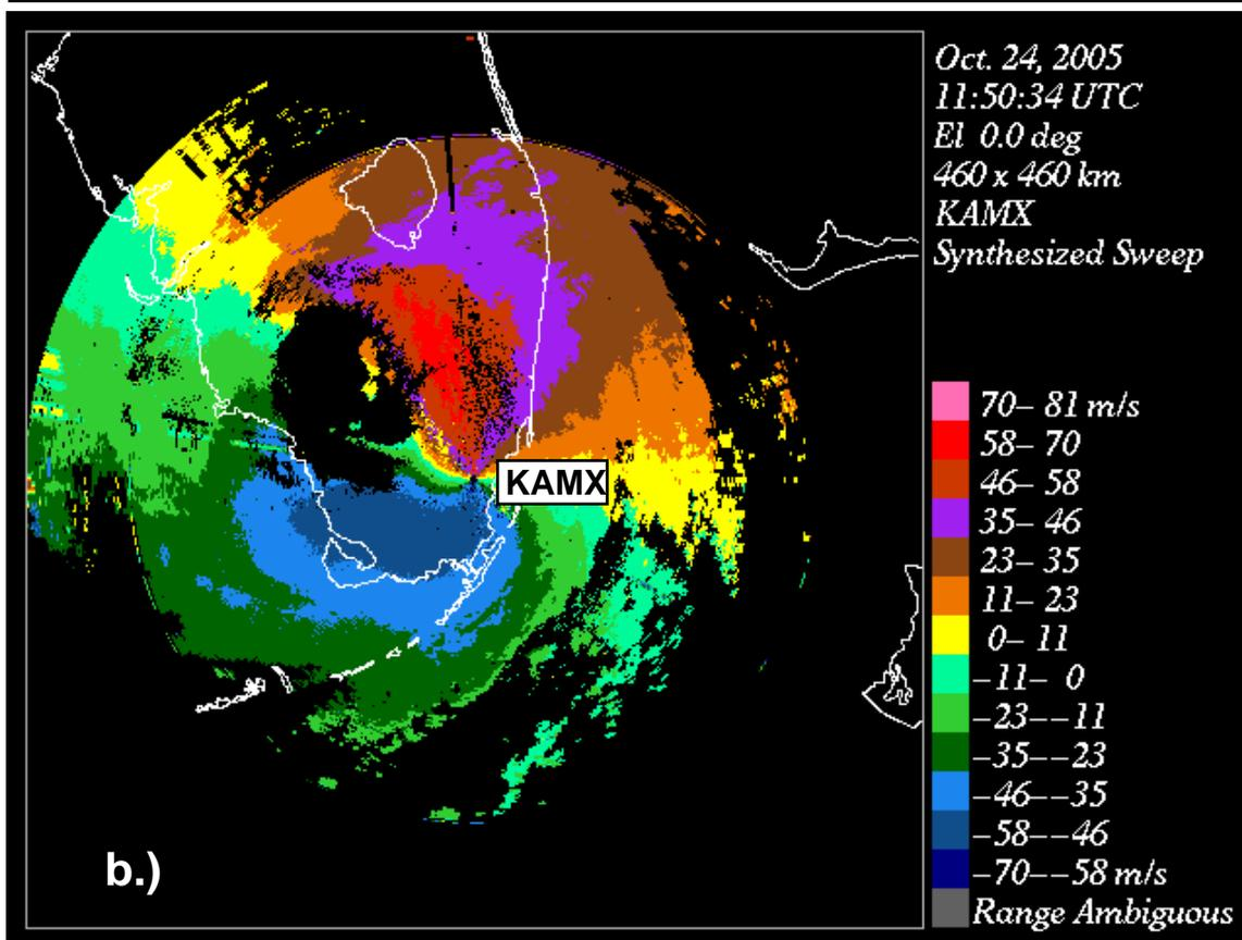
Figure 3. Radar images at 1150 UTC, 24 October 2005. Images from data synthesized from 0.5 degree sweeps. a.) Reflectivity and b.) Doppler velocity. Doppler Data dealiased. Green and blues indicate flow towards the radar and reds and oranges indicate flow away.
