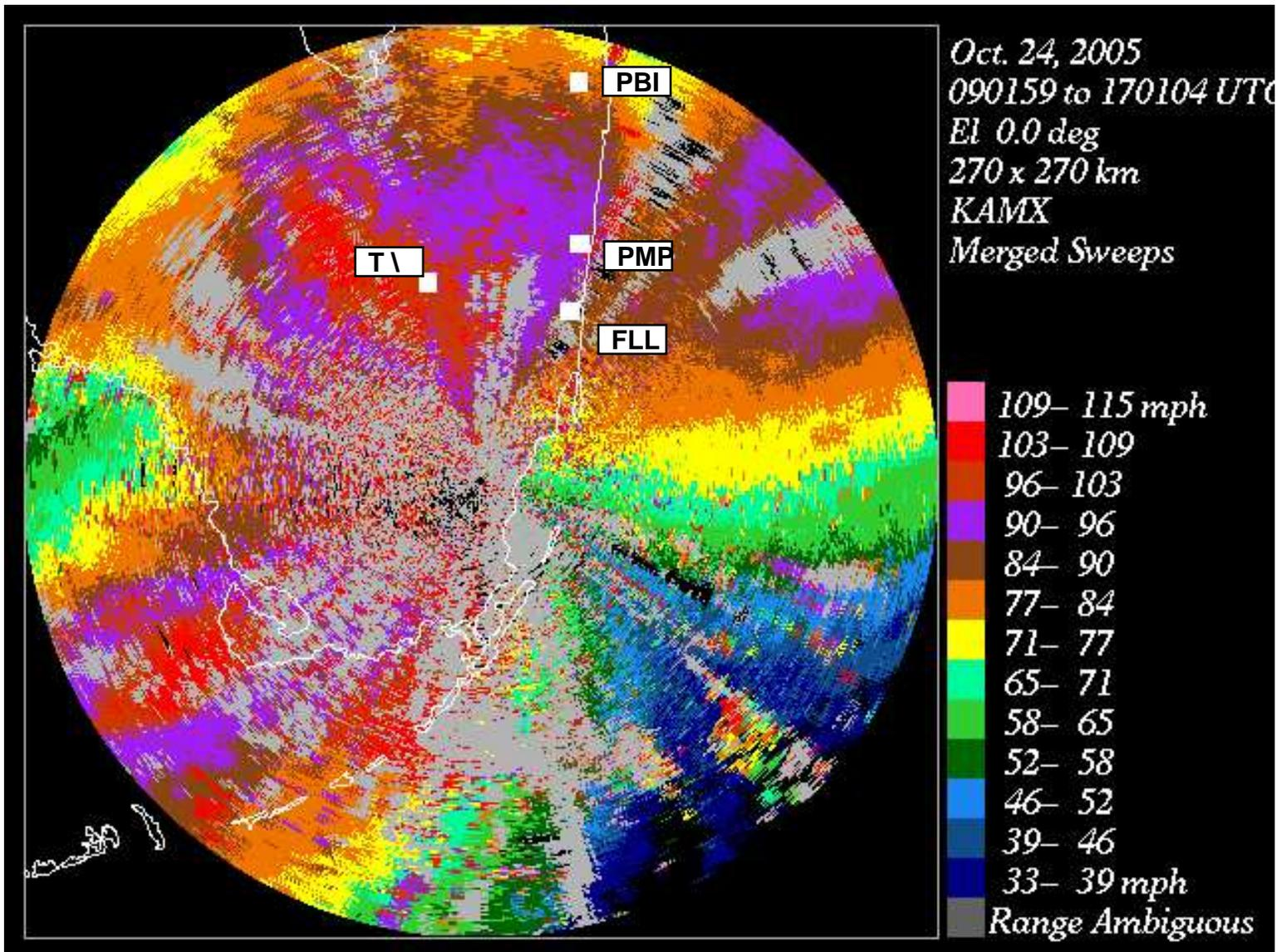
**Figure 5. Maximum Doppler velocities within 135 km of Miami WSR-88D for the period 0900 to 1700 UTC, 24 October 2005. Values displayed are absolute values reduced by a surface reduction factor of 70% to approximate sustained surface winds at 10m. T 1 is an FCMP tower and PBI, PMP and FLL are NWS ASOS sites..**
