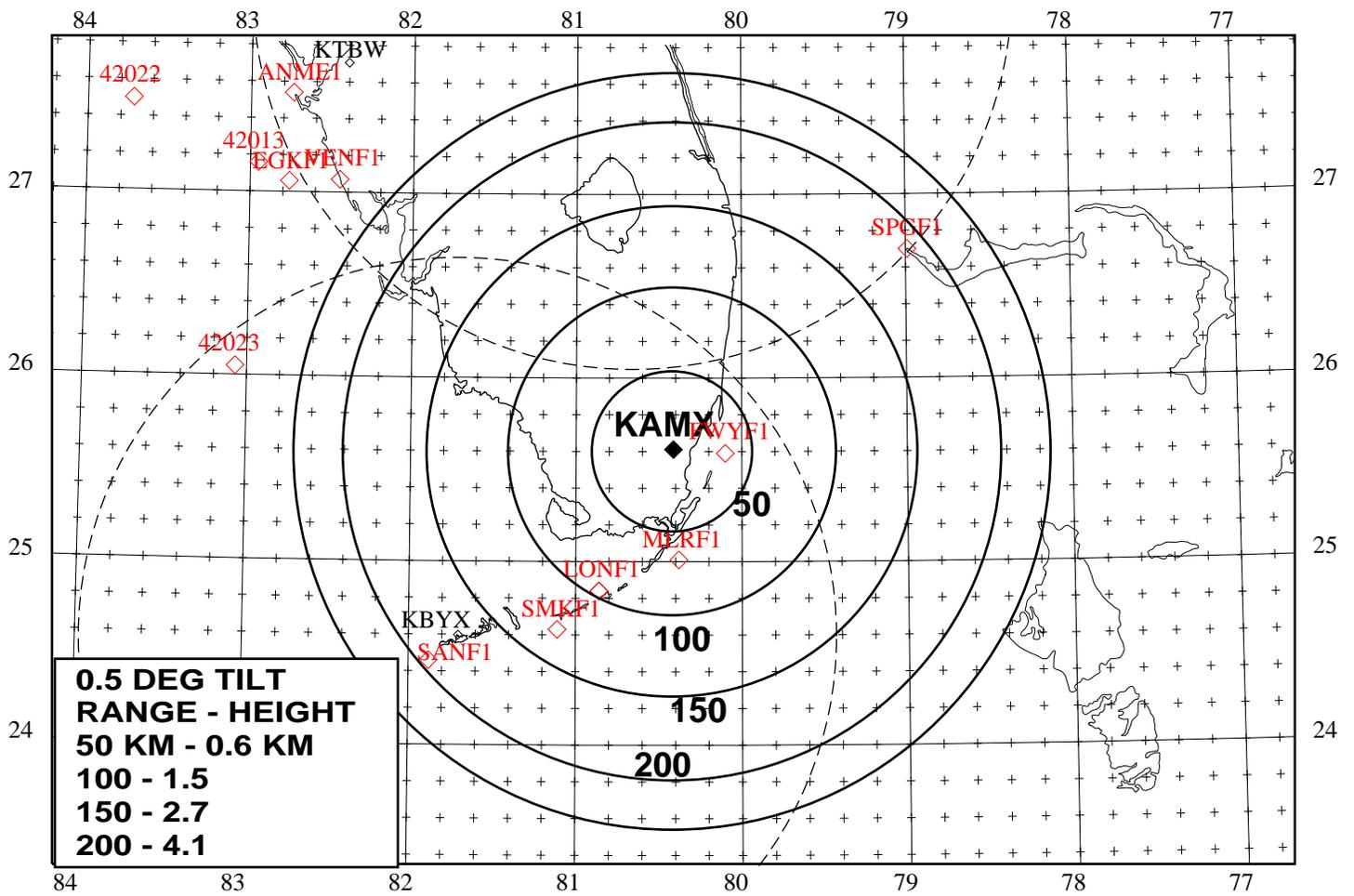
**Figure 2. Miami WSR-88D coverage. Table lists the beam midpoint height at different ranges.**
