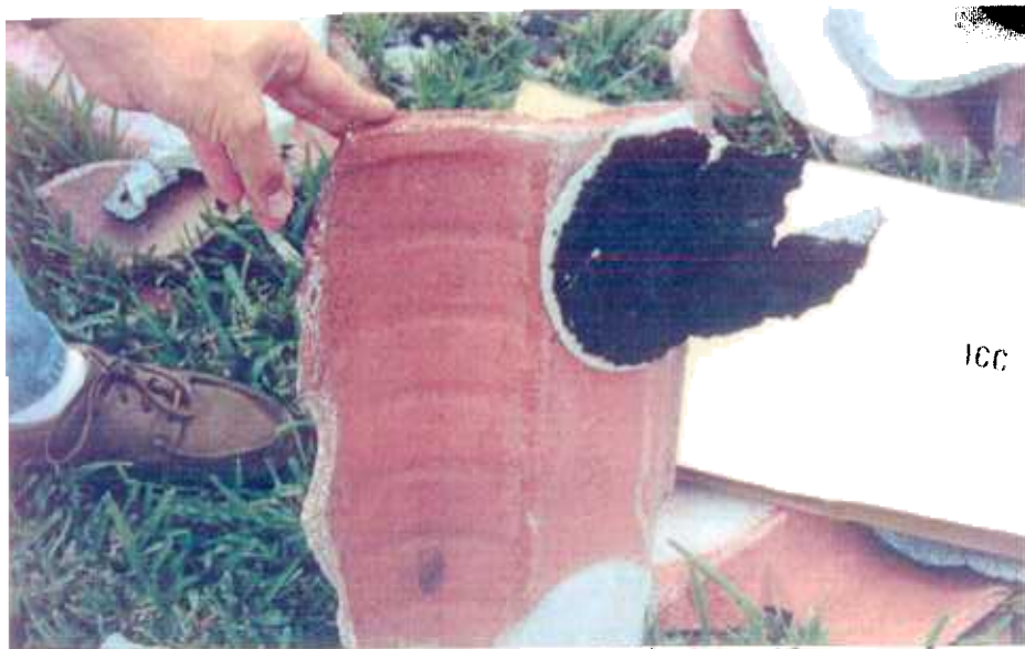
31. Tiles that bonded well to the mud failed along the roll roofing underlayment (Homestead).
