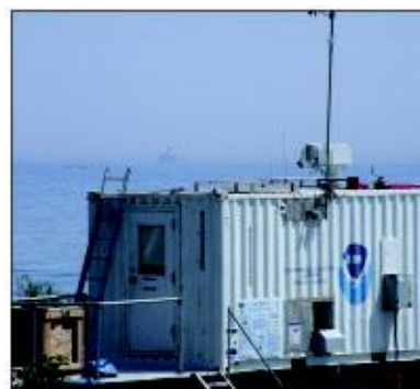
OAR - ETL - LIDAR - TEACO -ost High Power Doppler Lidar TEACO2 is a scanning atmospheric Doppler lidar that provides range-resolved measurements of radial wind speed and backscatter intensity.
