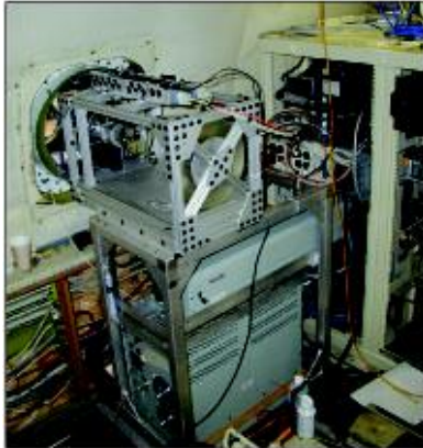
OAR - ETL - ABAEL Airborne Aerosol Lidar Backscatter lidar for aerosol detection on aircraft platforms.
