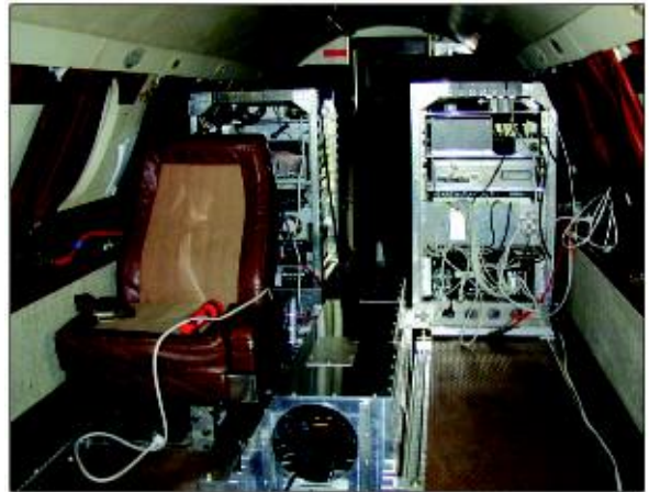
OAR - ETL - LIDAR - HRDL - ost High resolution Doppler lidar HRDL is a scanning atmospheric Doppler lidar that provides range-resolved measurements of radial wind speed and backscatter intensity. It is designed to make higher spatial and temporal resolution measurements in the atmospheric boundary layer.
