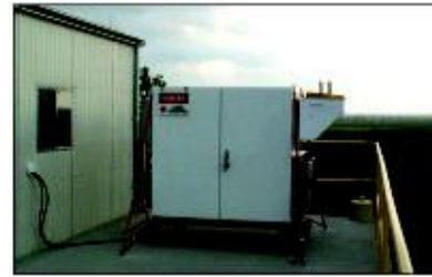
OAR - ETL - WVDIAL Compact Water Vapor DIAL Lidar This is a compact eye-safe autonomous lidar for profiling water vapor in the lower troposphere.
