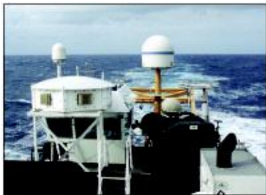
OAR - ETL - Windprofiler - RB Electronically-Stabilized Wind Profiler 915-MHz clear-air radar for measuring wind speed and direction from 150 - 3000 m altitude. System automatically compensates for platform motion.
