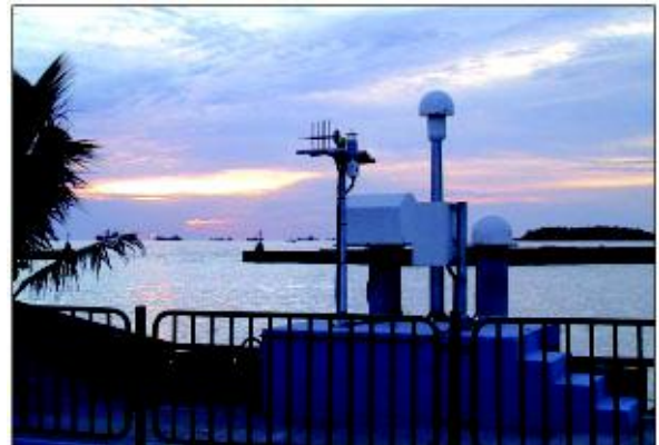
OAR - GSLN Global Sea Level Network GSLN stations are fixed platforms on islands and in the coastal zone that measure and report sea level information in real-time using geostationary satellites and the GTS.
