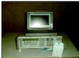
OAR - ETL - Rawinsonde - MW11 Rawinsonde - MW11 OAR - ETL - Rawinsonde - MW15 Rawinsonde - MW15 OAR - ETL - Rawinsonde - MW21 Rawinsonde - MW21 The Rawinsonde MW11, MW15, and MW21 observing systems consist of a sounding system manufactured by Vaisala. These systems measure temperature, relative humidity, pressure, wind speed and direction of the atmosphere. They use Global Positioning Systems (GPS) to determine wind speed and direction.
