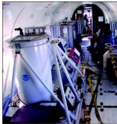
OAR - ETL - Airborne Ozone Lidar Airborne Ozone Lidar This system is a laser-based active remote sensor (LIDAR system) for measuring ozone concentration and aerosol optical backscatter in the lower troposphere.
