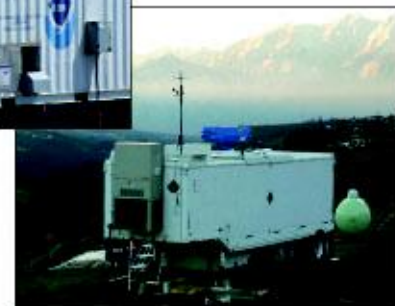
OAR - ETL - LIDAR - TEACO -ost High Power Doppler Lidar TEACO2 is a scanning atmospheric Doppler lidar that provides range-resolved measurements of radial wind speed and backscatter intensity.
