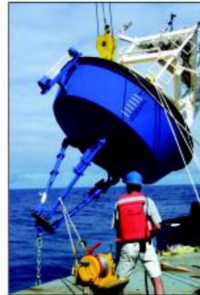
Deployment of Stratus 3 mooring off the northern coast of Chile.
