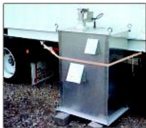
OAR - ETL - IRadiometer IR Radiometer Infrared radiation sensor for measuring temperature.
