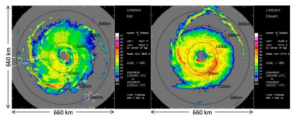
Fig.2. P-3 lower fuselage radar showing 25-40 dBZ circular convective bands in the environments of (left) 2010 Hurricane Earl (R=~200-250 km) at ~830 LST and (right) 2014 Hurricane Edouard (R=~150-300 km) at ~1300 LST. These circular outer band features are often coincident with TC diurnal pulses/waves and may be linked to the TC diurnal cycle.
