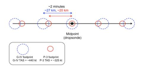
**Figure 3.** A schematic diagram of the flight path of the G-IV and P-3 aircraft during the module is provided. The red and blue circles indicate the P-3 and G-IV SFMR footprint size, respectively. The timing between successive locations in the figure is  $\sim 2$  minutes with the distance covered by each aircraft noted. This figure is not to scale as the footprint size is emphasized for visibility.
