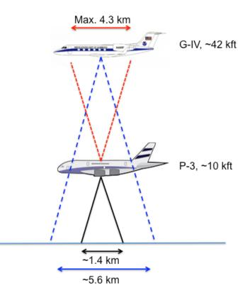
**Figure 1.** A schematic figure of the footprint coverage for the various SFMR instruments is provided. Also indicated are the normal operating altitudes of each aircraft. This schematic is not to scale.
