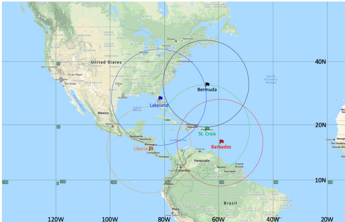
Figure D-1. Primary Atlantic operating bases and ranges (assuming ~2-h on-station time) for the P-3
