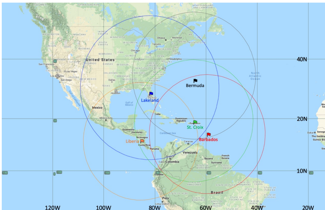
Figure D-2. Primary Atlantic operating bases and ranges (assuming ~2-h on-station time) for the G-IV
